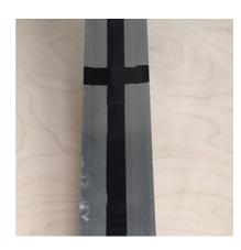
With TWEHA Blacken we have developed a black paint especially for this purpose. With the high demands for a durable adhesion to the aluminum and the (partly) creation of a durable bonding surface for the TWEHA adhesive systems as a requirement.
