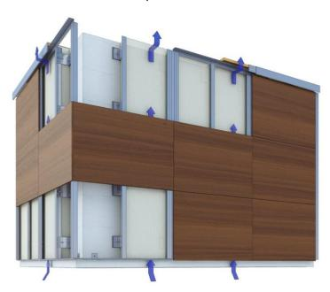
A ventilated rainscreen system features a continuous air space, open top and bottom, to encourage airflow and convective drying when water gets between the cladding and the exterior wall of building – whether due to wind-driven rain, bulk water shedding, or capillary action through porous cladding.
