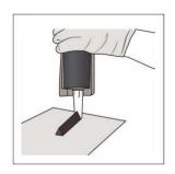
To obtain the prescribed glue width / thickness of at least  $12 \times 3$  mm, cut a standard nozzle in a 'V' shape of at least  $8 \times 8$  mm.
