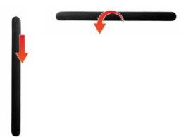
However, in the traditional mounting of cladding slabs with a vertical subframe the shear force runs parallel with the vertical adhesive bead, as we say along the strongest axe of the material (whole length of the adhesive bead). But in case of a horizontal adhesive bead shear forces will also occur perpendicular on the created adhesive bead, as we say along the weakest axe of the material (only the width of the glue bed).
